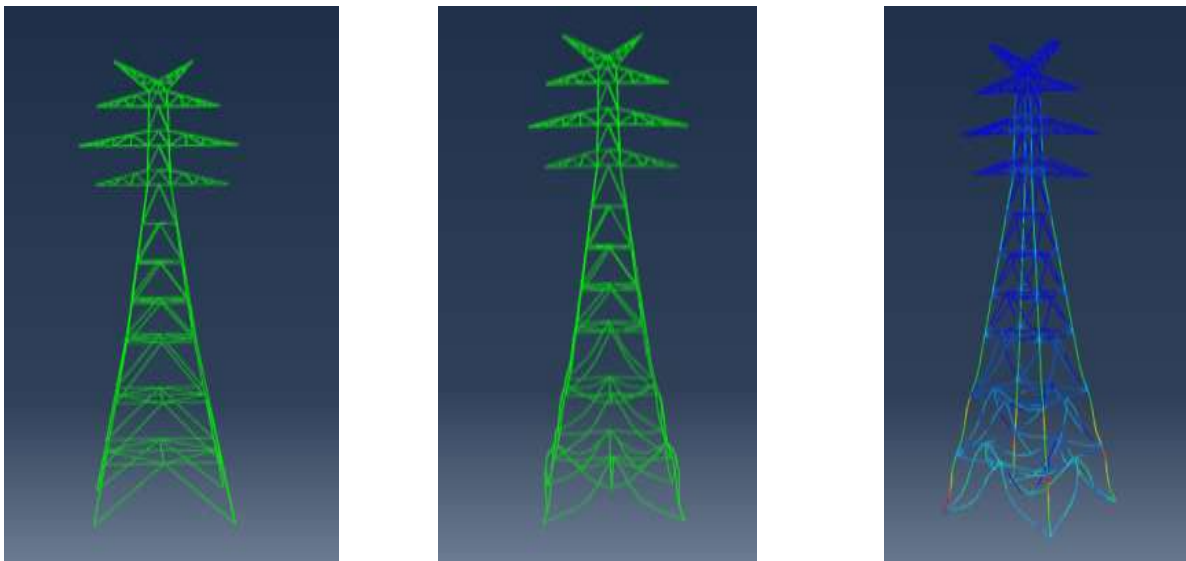
Figure (16) Pinned boundary condition of the supports
