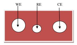
The above diagram shows the 3 electrode biosensor with working electrode, counter electrode and reference electrode. The 3 electrodes are dipped in bulk solution ,the bulk solution is phosphate buffer. Why phosphate buffer is taken, because of presence of phosphate in human DNA. This paper consists of mobilization and immobilization conditions of GODx enzyme
