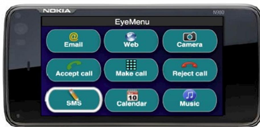
Figure : Eye Menu on the Nokia N900. While looking the display, a button is highlighted if it matches the eye position on the display. The highlighted button is ready to be “clicked” with a blink of the eye. In this example, the user is looking at the SMS button and the SMS keypad is launched by blinking the eye.
