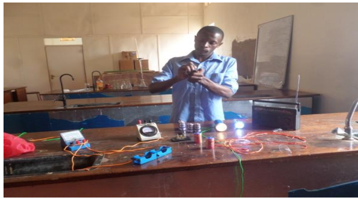
Figure 1: Shows how the initial Voltages and Currents of the battery cells were found
