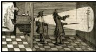
Figure (7) Early drawing of a magic lantern in use from Zahn's Oculus Artificialis Teledioptricus Sive Telescopium (1702). Rakow Library collection
