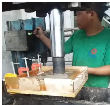
Figure 3: Pressing of the board with the use of hydraulic press then clamping the board.
