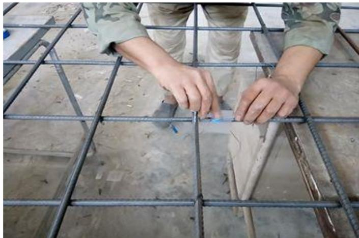
**Fig 10: Installation of the Strain Gauges to the Steel and GFRP Reinforcement**
