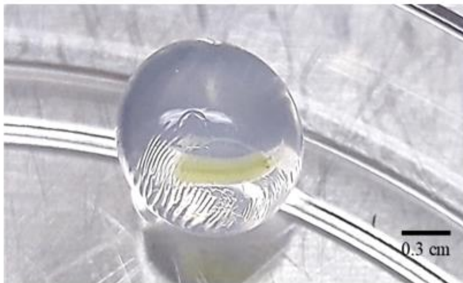
Fig 1. Bead was roundly formed, firm and in a good shape after 4% of sodium alginate left hardened in 0.1M calcium chloride dehydration for 30 – 45 minutes
