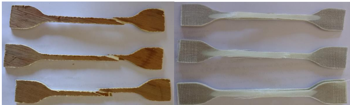
Fig.4.1: Tensile Fractured specimens of Areca nut fiber and Areca nut fiber & Glass hybrid composite
