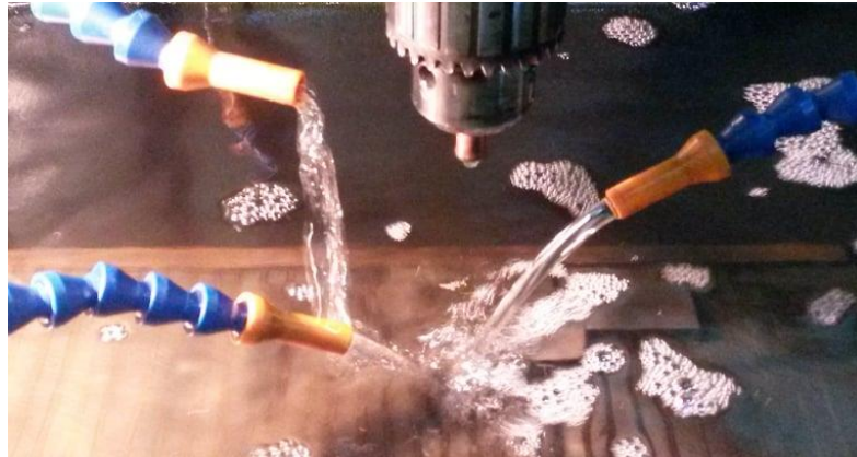
Fig. 7 Gap setting between electrode and workpiece
