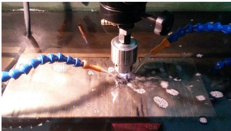
Fig. 8 Jet flushing nozzle setup
