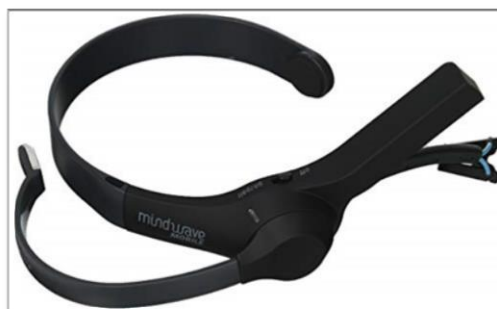
Figure 4: Neurosky Mindwave device
